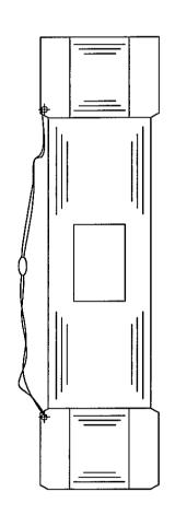
GENERAL DESCRIPTION: THESE PRECISION-MADE INLINE RELIEF VALVES FEATURE REPLACEABLE DISC ASSEMBLIES AND NOZZLES OF STAINLESS STEEL, STELLITE OR PLASTIC INSERTS WITH STAINLESS STEEL BODY, BASE AND BONNETS. PERFORMANCE IS BUBBLE TIGHT AFTER REPEATED OPERATIONS. MODEL 5000, 5100, AND 5200 VALVES ARE HIGHLY SUITABLE FOR HYDRAULIC, AIR, AND GASEOUS SYSTEMS.
