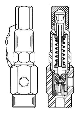
GENERAL DESCRIPTION: THESE COMPACT SAFETY RELIEF VALVES ARE DESIGNED TO HANDLE DRY, CLEAN GASES FROM HYDROGEN TO NITROGEN WITH BUBBLE TIGHT PERFORMANCE AND CONSISTENT REPEATABILITY UP TO PRESSURES OF 15,000 PSIG. THESE VALVES CAN BE MADE OF ANY MATERIAL CLASSES UPON REQUEST.
